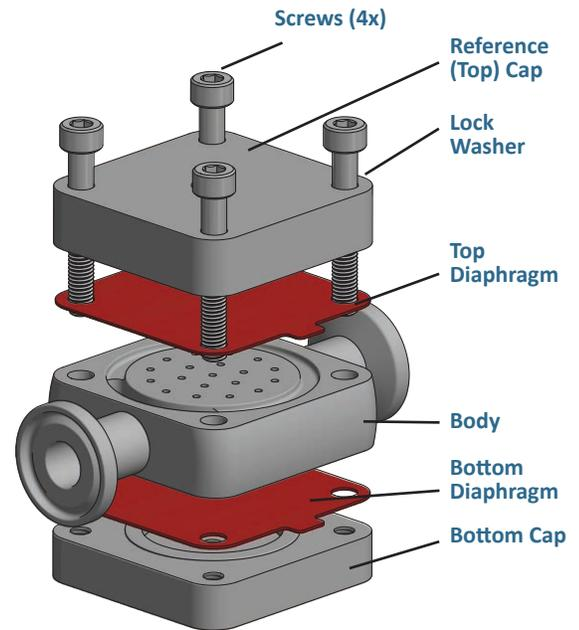
Figure A: FDO4 Exploded View
